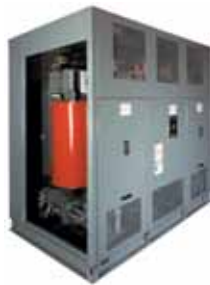
Uni-Cast II transformer Cast coil primary encapsulated secondary kVA sizes: 500 kVA – 3,000 kVA Primary voltage classes: 2.4 kV – 34.5 kV
