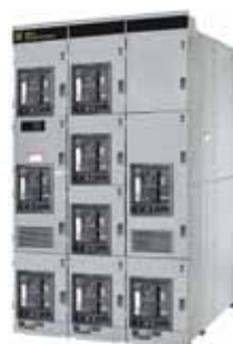
QED-6 Power-Style® switchboard Masterpact NT and NW power circuit breaker Bus ratings up to 5,000 A, 600 V and below
