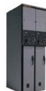
Motorpact medium voltage motor controller Power 2.4 kV – 6.9 kV Max. 50 Hz – 60 Hz Bus ratings up to 50 KA Control: 120 V, 60 Hz; 110 V, 50 Hz
